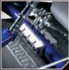
Split front axle beam with adjustable machined billet alloy chassis clamp
