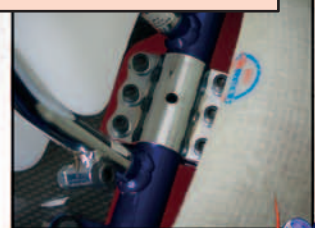
SPLIT FORWARD CROSS RAIL WITH OPTIONAL ADJUSTABLE CHASSIS CLAMP
