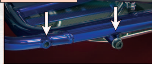
UNIQUE SHORT/LONG-PEDAL MOUNTING OPTION TO SUIT DIFFERING HEIGHT DRIVERS
